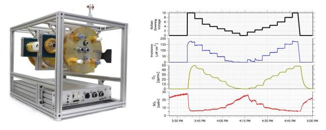
Time series from an example OH exposure calibration experiment using  $SO_2$  as a reactive tracer species. The dimming voltage applied to UV lamp ballasts is stepped from 0-10 VDC, which varies the UV irradiance and the ozone mixing ratio in the PAM chamber.
