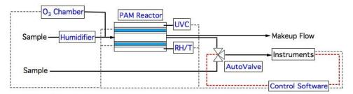
Typical setup for measurements incorporating PAM reactor. Control software facilitates data- logging at 1 Hz and automated control with event sequencing for unattended operation (dashed grey=analog input/output; dashed red=digital input/output)
